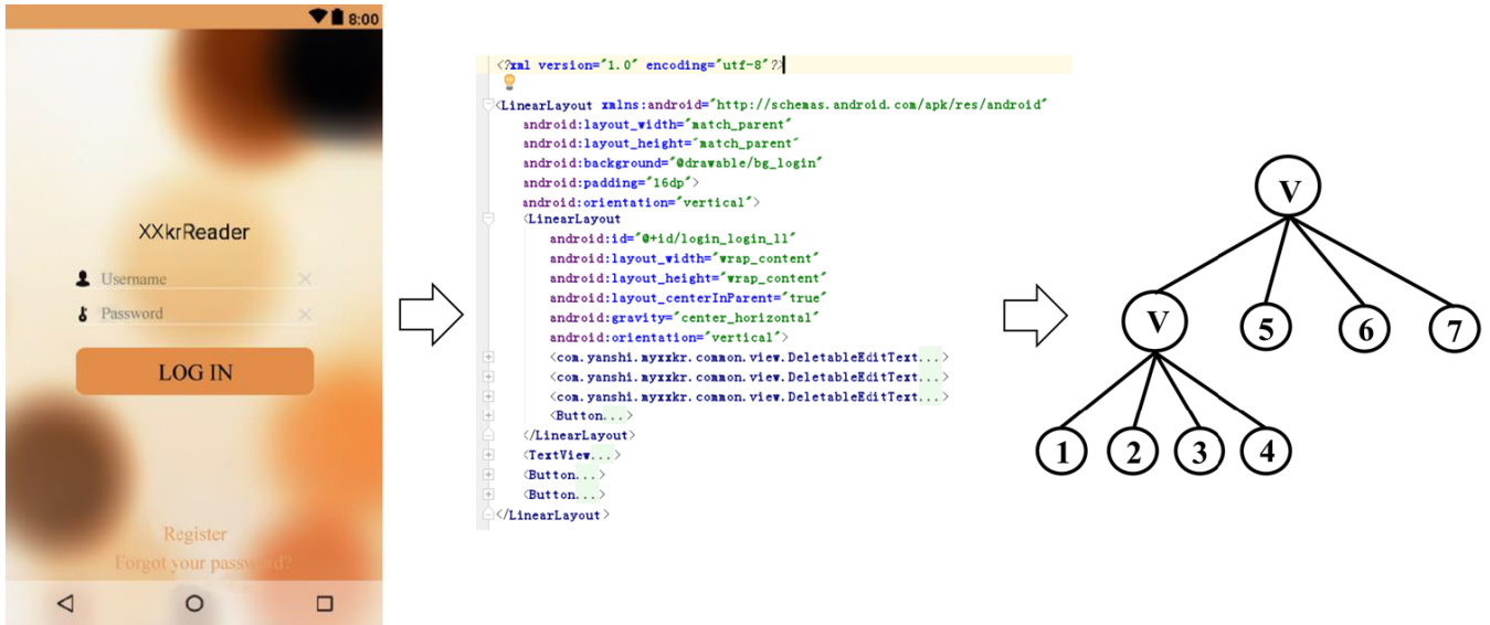
FIGURE 1. A user interface, its corresponding code and the visual-representation tree. In the visual-representation tree, the “V” label of an internal node indicates that its children are organized in a vertical layout, and the numbers in the leaf nodes indicate the indexes of the widgets they represent.
