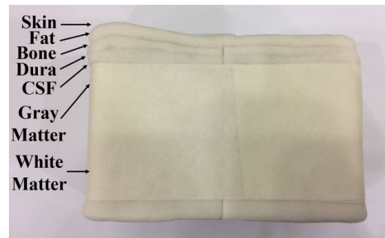
FIGURE 8. The fabricated seven-layer brain phantom.
