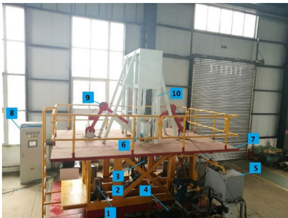
FIGURE 20. The equal proportional reduction model of the crane type active and passive combined heave compensation system. 1 Stroke Column of, Operating Platform, 2 Traveling Block, 3 Compensation Cylinder, 4 Circulating Filter Cooling Refueling Device, 5 Oil Tank, 6 Crane, 7 Offshore Operating Platform, 8 PLC Control Cabinet, 9 Active Cylinder of Rocker Mechanism, 10 Guide Rail of Crane.
