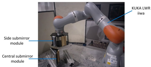
FIGURE 15. Experiment setup for submirror assembly.
