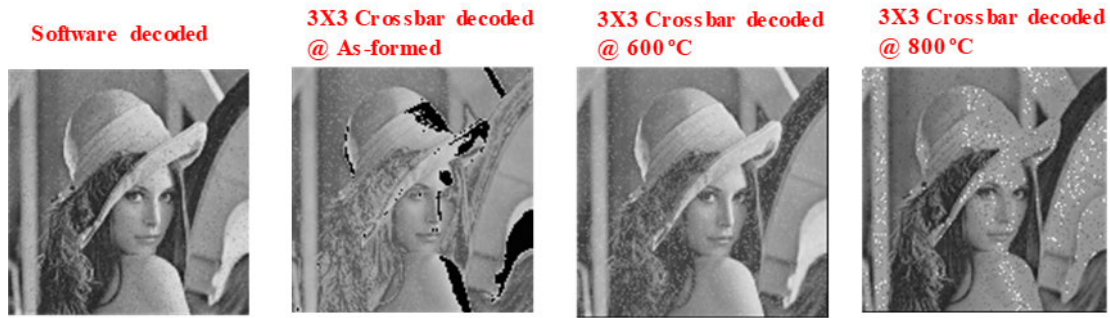
FIGURE 15. Output of decoded image through different crossbars.
