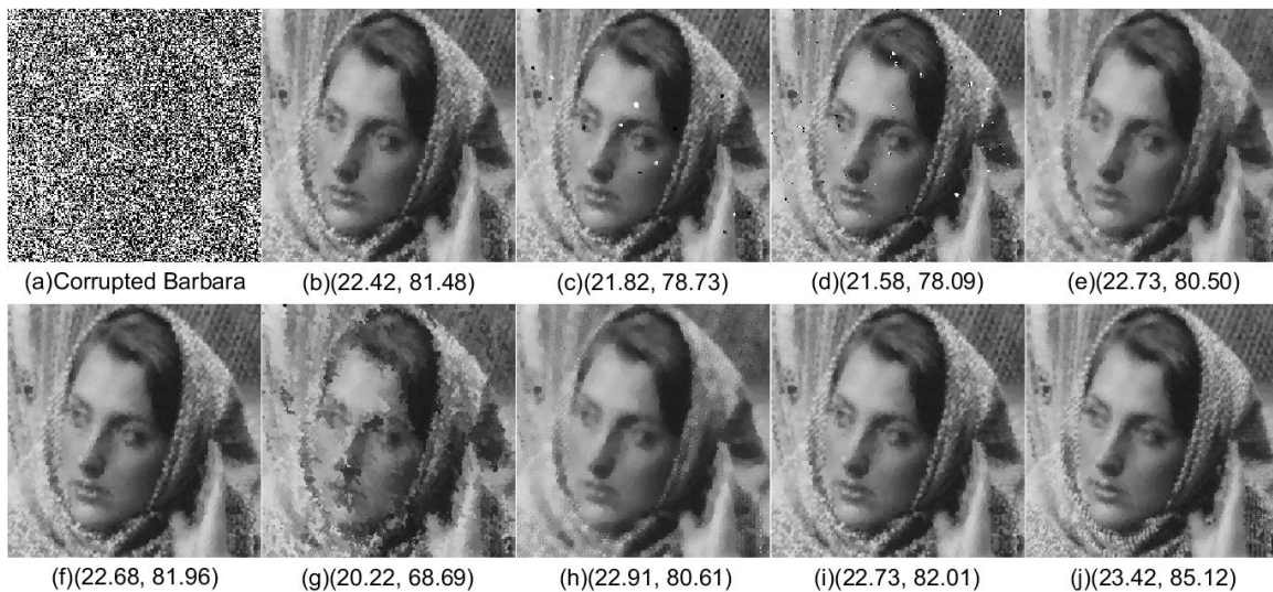
FIGURE 11. Recovery results of image Barbara with 80% impulse noises.(a) Zoomed-in local part of Barbara with impulse noise; Results of (b) DAMF; (c) NDBINF; (d) PVGF; (e) ADWMF; (f) RBF; (g) SVMFF; (h) NAISM; (i) INLM; (j) ASWMF.
