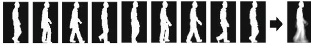
FIGURE 8. A representation of extracted GEI from the entire sequence of silhouette gait from the study [12].
