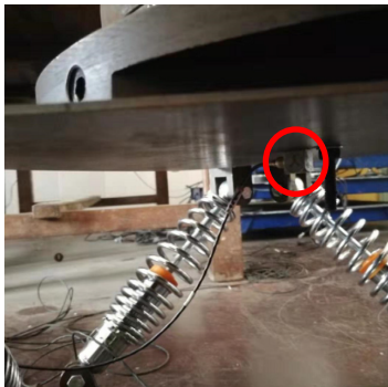
(b) The acceleration sensor arranged at the upper platform
