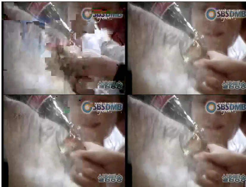
FIGURE 11. One frame from DMB video sample no. 1, Top-left: errors in Cell 1, top-right: errors in Cell 2, bottom-left: errors in Cell 3, bottom-right: errors in Cell 4 (Error rate = 1.33 \times 10^{-4} ).
