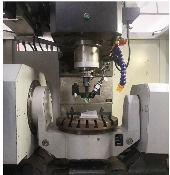
FIGURE 16. Contact measurement on the CNC machine tool.
