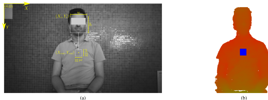
FIGURE 2. Capture examples of the IR feed and Depth Point-Cloud from the preliminary tests (not the actual setup), with the metrics used to compute the ROI depicted in the IR feed and the final ROI represented as a blue square in the Point-Cloud. The ROI used to extract the respiratory signal (blue square) from the Depth Point-Cloud can be appreciated in (b).
