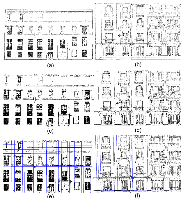
FIGURE 11. Qualitative comparison. (a) The boundary points of facade point cloud 2. (b) Removing the boundary points that are close to the convex hull of facade point cloud 2. (c) The splitting result that is obtained using the method of Peethambaran and Wang [8]. (d) The boundary points of facade 3. (e) Removing the boundary points that are close to the convex hull of facade 3. (f) The splitting result that is obtained using the method of Peethambaran and Wang [8].
