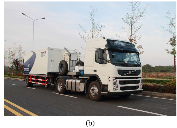
FIGURE 2. The laser dynamic deflectometer. (a) The method of continuous dynamic deflection measurement. (b) The vehicle measuring system of the laser dynamic deflectometer.
