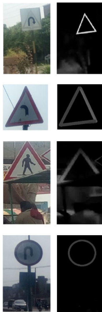
FIGURE 10. Samples containing standard and with degradations present on the outer rim of the traffic sign detected with our proposed flexible mixture model based segmentation technique.
