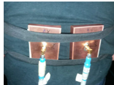
FIGURE 31. Two proposed UWB antennas placed on the belly area for on-body measurement scenario.
