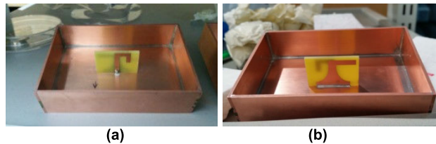
FIGURE 9. Antenna prototype of the studied UWB antenna in (a) Front and (b) Back views.
