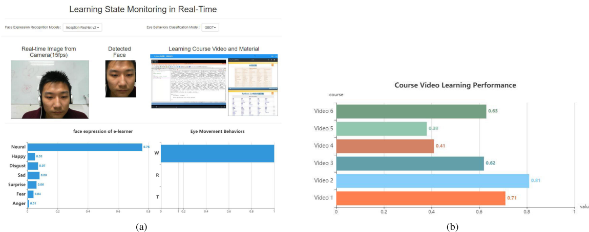
FIGURE 11. Visually recognizing learner’s engagement from three facets. (a)Monitoring learner’s facial expressions, Eye movement behaviors in real-time. (b)Monitoring learner’s performance on each short video course.
