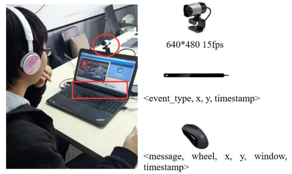
FIGURE 6. Experimental setups in lab environment.
