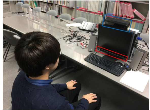
FIGURE 2. Environment of the experiment. A blue rectangle and a red rectangle indicate a Web camera for OpenPose and Tobii Eye Tracker 4C, respectively.
