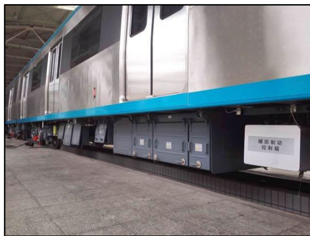
FIGURE 23. The photo of the traction system of Beijing Subway Line 14.
