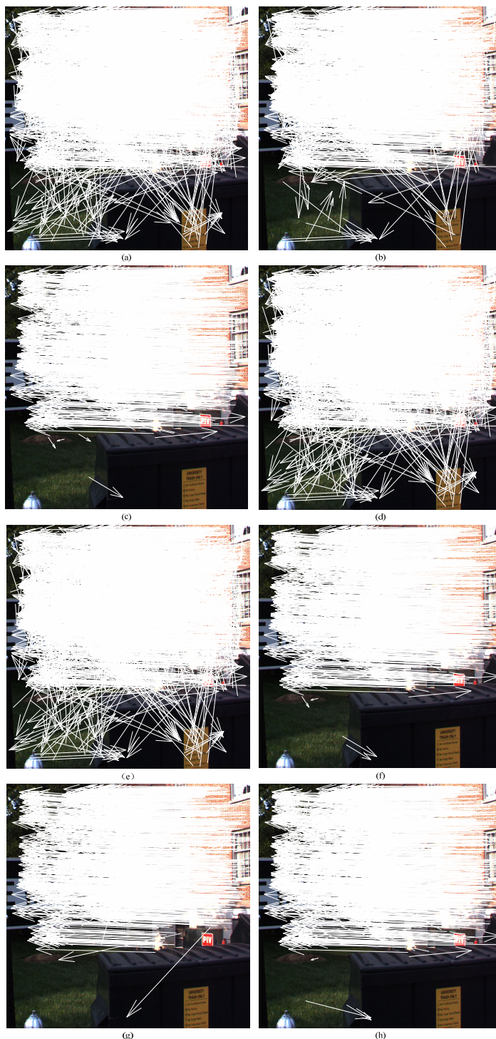
FIGURE 8. Robustness comparison of seven different methods with Scene2. (a) Initial correspondences; (b) Inliers obtained by M-estimator; (c) Inliers obtained by LMedSeig; (d) Inliers obtained by RANSAC; (e) Inliers obtained by FNS; (f) Inliers obtained by SDO; (g) Inliers obtained by L2E-LSC; (h) Inliers obtained by the proposed method.
