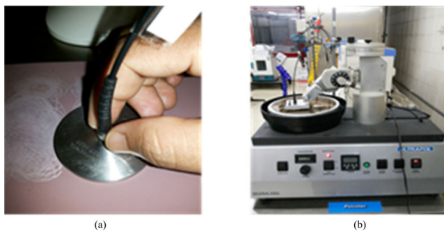
FIGURE 3. Steps of polishing process (a) first stage: manual, dry polishing (b) second stage: using polishing machine, wet polishing.
