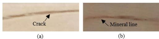
FIGURE 2. Crack and mineral line on the surface of the birch veneer: (a) Crack and (b) Mineral line.
