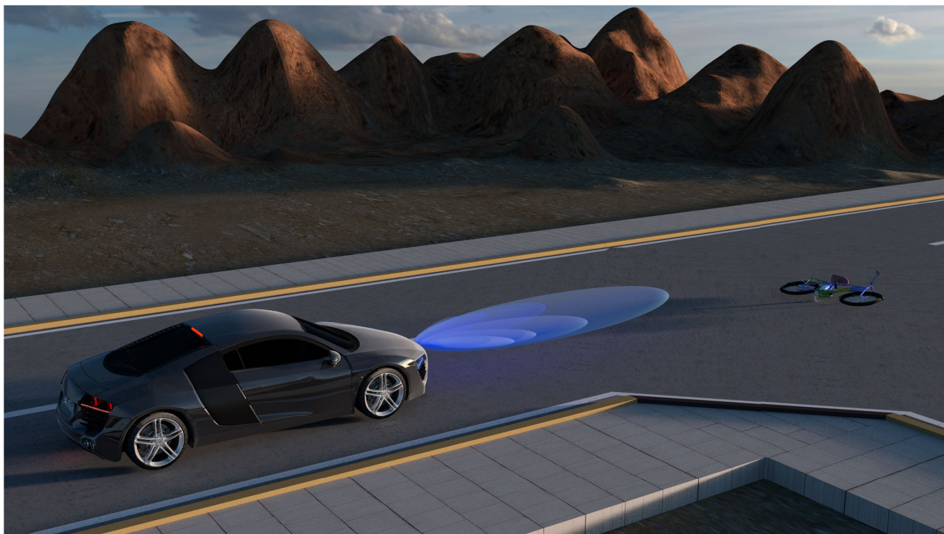
FIGURE 1. Representation of a symphotic edge detector deployed on a car. The device is mounted on the front and it detects the presence of obstacles ahead on the road.
