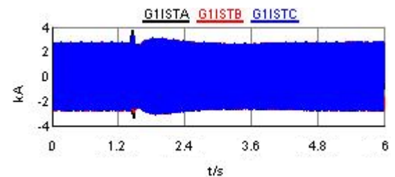
FIGURE 19. Stator current response curve of improved control strategy.
