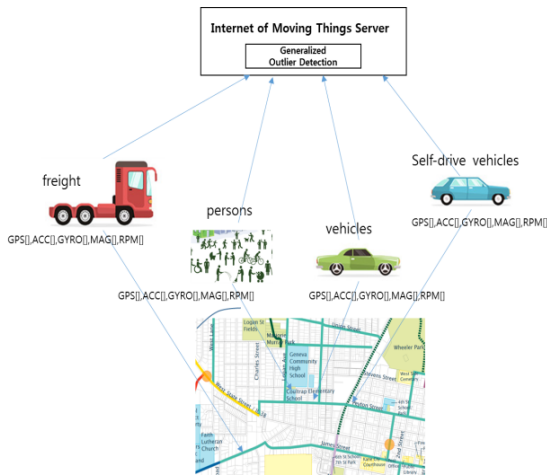
FIGURE 1. An example of the Internet of Moving Things with different moving things, such types of things contains many GPS data, accelerometer data, gyroscope sensor data, magnetometer data, and RPM sensor data, etc.
