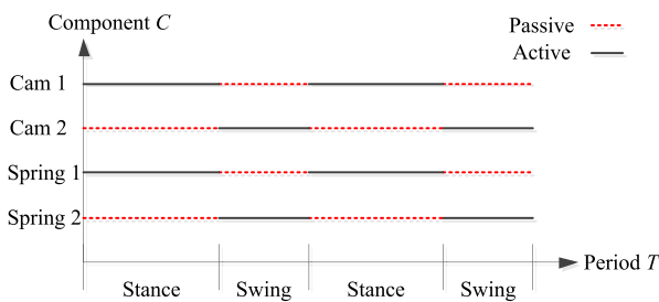
FIGURE 4. The timing diagram of operations for each conjugate cam and spring.
