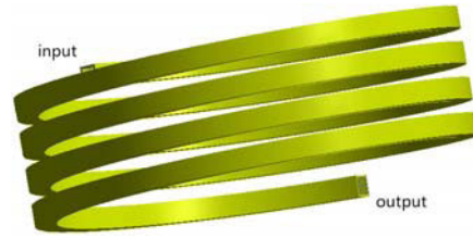
FIGURE 6. 3D model of the cooling channel.
