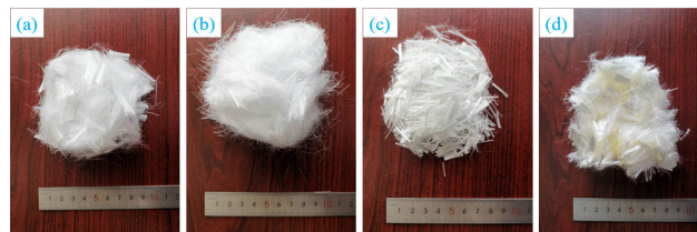
FIGURE 3. Four kinds of fibers: (a) polypropylene; (b) polyacrylonitrile; (c) glass; (d) polyvinyl alcohol.
