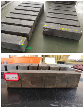
FIGURE 4. Photos of rectangular fiber reinforced CTB samples.
