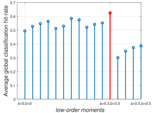
FIGURE 12. Average Global classification hit-rate for the considered GSNR range, for distinct fractional lower-order moments, obtained by the FLOCAF-based architecture.
