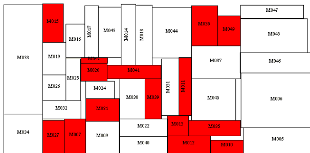
FIGURE 5. Floorplanning for circuit ami49 layer 1 (bottom layer).
