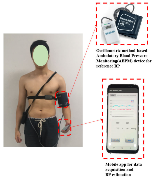
FIGURE 6. Setup of daily BP monitoring. Subjects wore the developed device and reference oscillometric method-based ABPM carrying the mobile phone that collects the data, shows processed signals, and estimates BP online. They were asked to behave freely during a day, without particular regulations on any type of activity.
