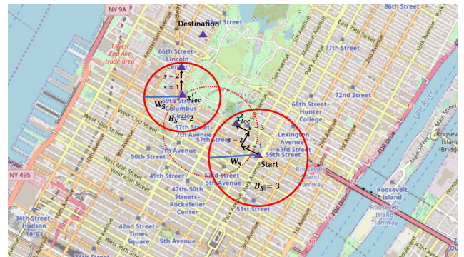
FIGURE 4. LCWSA strategy: The cloud server will provide a part of the route within a circle every W_S period.
