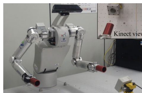
FIGURE 17. Peg-in-hole assembly system guided by robot with Kinect depth camera [130].
