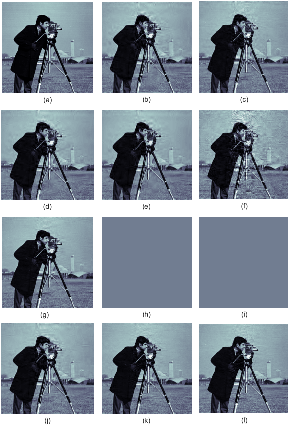
FIGURE 24. Reconstruction images of different algorithms under Cameraman image condition. (a) Original image; (b) OMP; (c) StOMP; (d) SP; (e) CoSaMP; (f) StoGradMP; (g) SAMP, s = 1 ; (h) SAMP, s = 5 ; (i) SAMP, s = 10 ; (j) Proposed, s = 1 ; (k) Proposed, s = 5 ; (l) Proposed, s = 10 .
