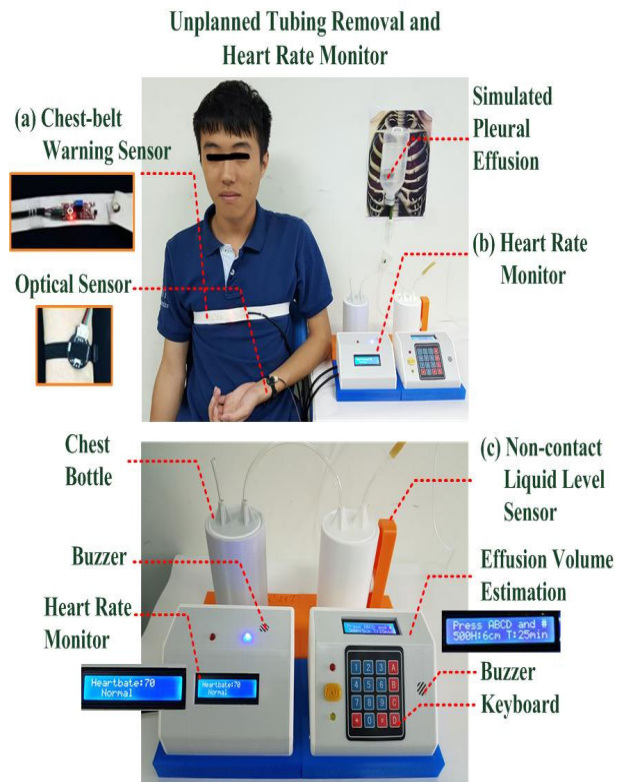
FIGURE 5. Implementation of the smart drainage monitoring system. (a) Detection of unplanned tubing removal, (b) monitoring the heart rate (physiological signal), and (c) estimation of effusion volume.
