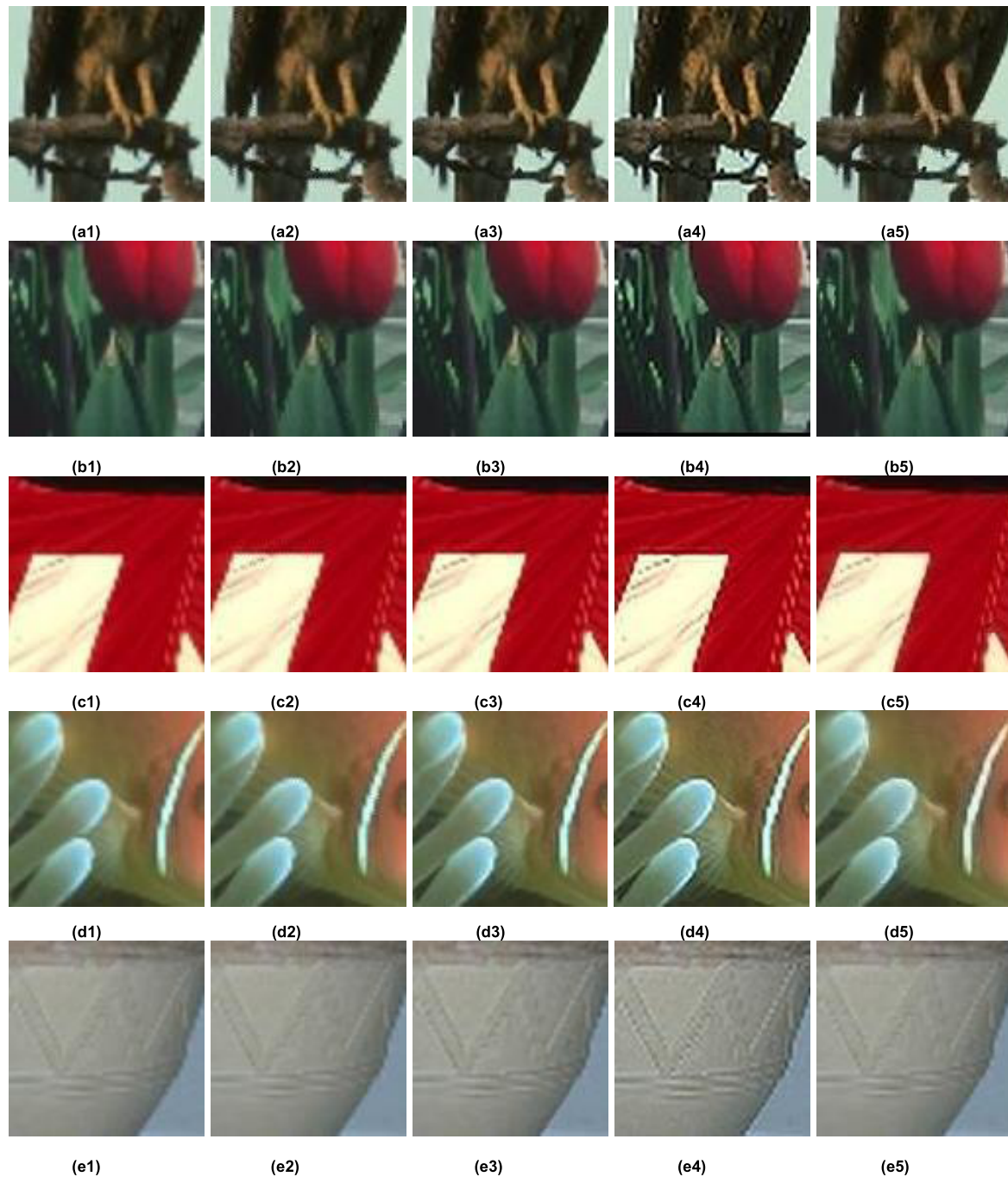
FIGURE 9. Cropped regions after upscaling ( \times 2 ): (a1)-(e1) Bicubic, (a2-e2) NEDI, (a3-e3) ICBI, (a4-e4) SL-ASR, and (a5-e5) Proposed.
