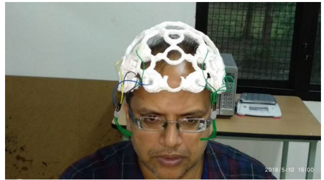
FIGURE 3. Signal acquisition using EEG sensor [21].
