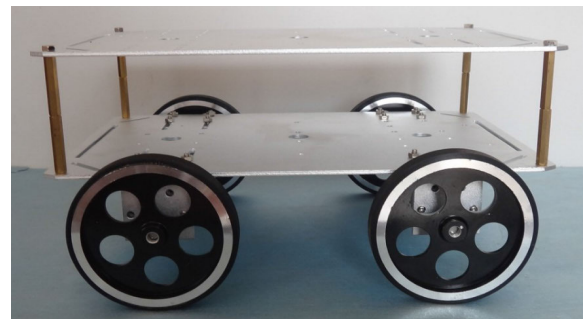
FIGURE 4. The overall size of the system is 30*20*20 cm, and the diameter of the wheel is 9.5 cm.
