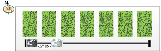
FIGURE 9. The system moves at a constant velocity from east to west along the path of the greenhouse, and the data are collected every 30 seconds.
