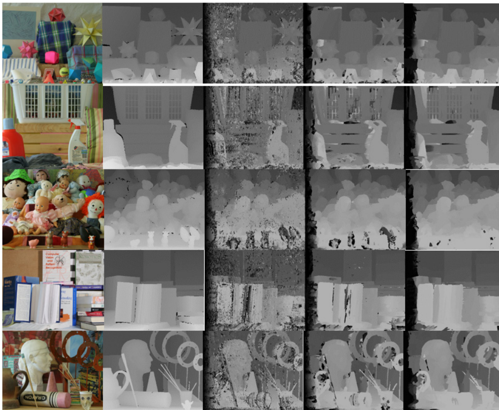
FIGURE 6. Results of the proposed stereo matching method. First column images are the color images, second column images are the ground truth images, third column images are the results of the bilateral cost aggregation, fourth column images are the results of the guided cost aggregation, and final column images are the results of the proposed method.
