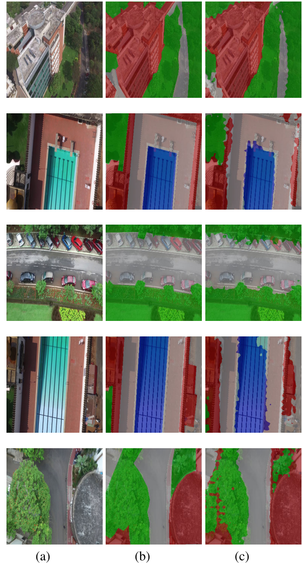
FIGURE 22. (a) Original image. (b) Ground truth image. (c) Semantic segmentation results by applying DeepLabV3+.
