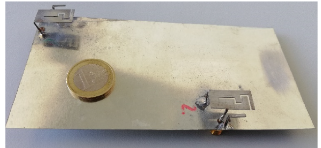
FIGURE 21. Fabricated prototype of double dual-band slotted PIFAs with the best isolation between the 2 elements.
