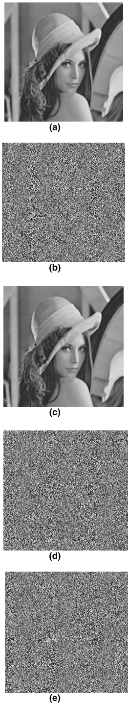
FIGURE 10. Image transmission of cross-layer security system. (a) Original image (b) image after data encryption (c) matched decoder/ correct AES (d) matched decoder/wrong AES (e)unmatched decoder/ correct AES.
