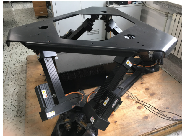
FIGURE 7. The experimental Stewart platform.
