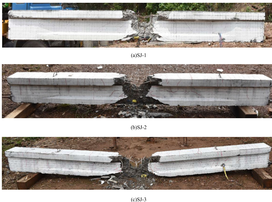
FIGURE 8. The damage condition in mid-span.
