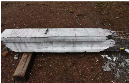
FIGURE 16. Left half span crack distribution of SJ-2.
