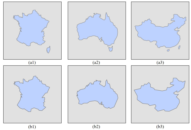
FIGURE 14. Experimental data for map outline design. (Group a: Original data; group b: Data after generalisation).
