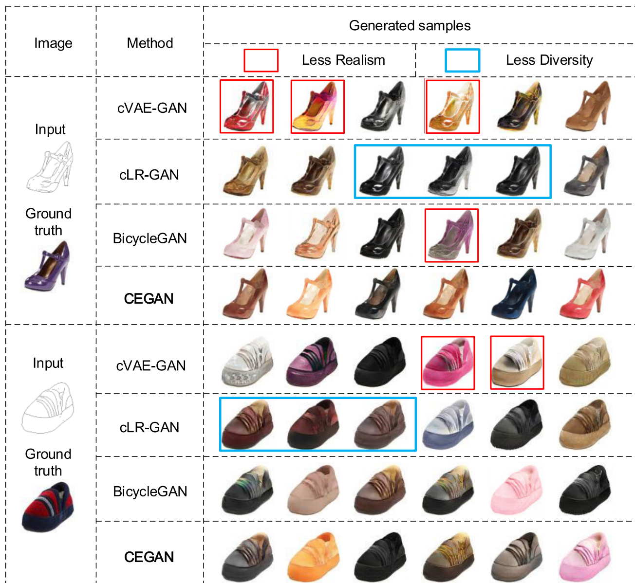
FIGURE 5. Qualitative comparison results. Comparison of randomly generated samples from different methods on the Edges–shoes dataset. Under the situation of the same input, the outputs of cVAE-GAN are diverse but not realistic (marked by red rectangle). The cLR-GAN produces realistic images while it is at the expense of diversity (marked by blue rectangle). BicycleGAN generates better outputs than the two methods, but the results from our CEGAN show the most realistic and diverse results.
