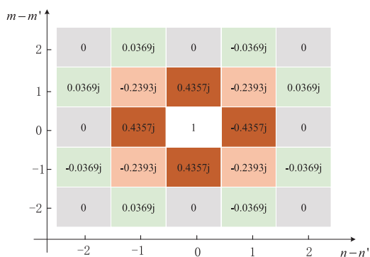
FIGURE 7. Imaginary interference ju_{m,n}^{m',n'} in the FBMC-OQAM using the Hermite filter with an overlapping factor of 4.
