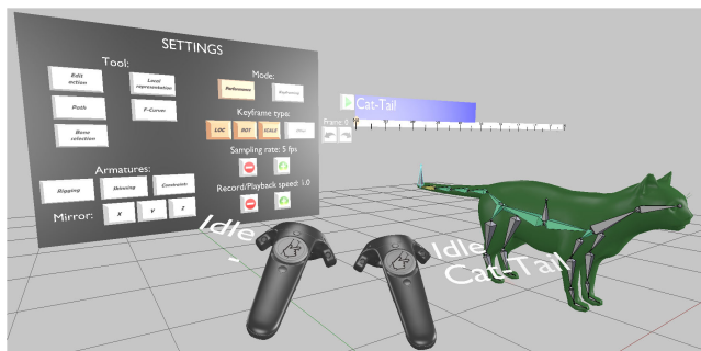
FIGURE 2. First-person view of the VR Blender immersive interface during user interaction; on the left side, widgets introduced to manage armature deformation-based animation tasks are shown. More information on other elements can be found in [9].
