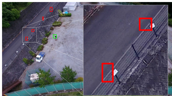
FIGURE 9. Example of 4 false positives, in red, detected along a fence in the surveillance field test. The fifth detection, in green, is a true positive.
