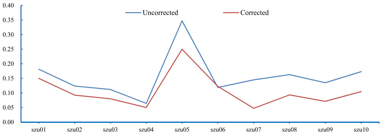
FIGURE 7. Comparison of the corrected and uncorrected over-water point cloud error in the outer precision.
