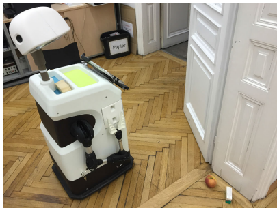
FIGURE 6. Objects which are too close to a wall or a fixed obstacle should not be grasped.
