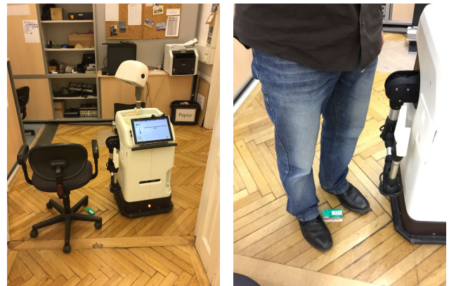
(a) A chair blocking the object. (b) A user blocking the robot arm.
